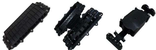
OSCH-120 Fiber Optic Splice Closure — Inline closure molded from ABS plastic for reliable splicing and distribution of various optical cables in access and distribution networks. It provides 4 round cable in/out ports supporting cable diameters from Ø7 to Ø18 mm. A mechanical sealing structure filled with sealing compound enhances environmental protection, and the closure is re-enterable—it can be opened after sealing for inspection or expansion.
