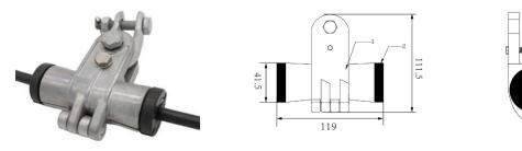
Technical data sheet for our Suspension Hardware designed specifically for spans of up to 150 meters, featuring part number OFT-SCCS-XXYY. This document provides comprehensive details regarding the specifications, features, and applications of this product. Developed to meet the rigorous demands of suspension applications, the OFT-SCCS-XXYY offers robust construction and reliable performance.
