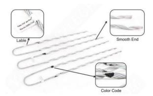
The OFT-PGG XX7 and OFT-PGG XX9 preforms are made up of 3, 4, 5 and 6 powerful helical ASTM A36 steel wires to evenly distribute the gripping force and tension, their anti-corrosion process is based on the ASTM 123 hot-dip galvanized standard. The OFT-PGG XX7 and OFT-PGG XX9 is designed for the perfect anchoring of ADSS and ASU cables in the deployment of FTTX networks.
