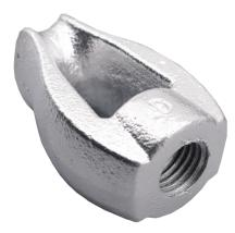
Thimble eye Threaded 5/8" Nut Hot dip Galvanized OFT-NTE58, it is used to attach to through bolts or to the threaded end of straight bolts or angled thimbles for side stays. Forged galvanized steel. Nuts are contoured to minimize tie rod bending and twisting spacing.
