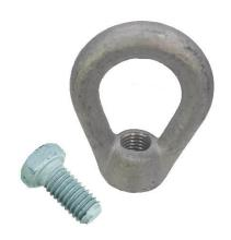
Eye Nut Hot Dipped Galvanized 5/8" UNC with 01 Bolt UNC 5/8" UNC OFT-EYN58-B, it is used to attach to through bolts or to the threaded end of straight bolts or angled thimbles for side stays. Forged galvanized steel. Nuts are contoured to minimize tie rod bending and twisting spacing.
