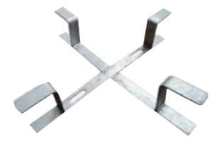
The rest cable stand is used in collecting reserved optical cable on the connecting tower(pole), on strain tower(pole) generally. The cable storage assembly shall be used together with joint box.
