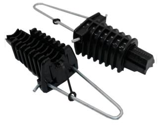
These anchoring clamps are made of an opened conical fiberglass-reinforced body, plastic wedges, and a SS201 bail. The anchoring clamps allow for easy and quick securing of  $\Phi$  6 to 9 mm conductors.
