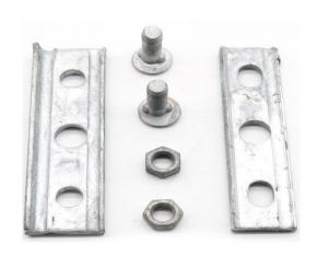
**The OFT-C3BCS** 2 Bolt Cable Suspension Clamp is used with through bolts to serve as clamping member. This Flat 3-hole clamp securely grips messenger strand to pole, it uses a nut and square washer that is used between the clamp and pole for proper spacing.
