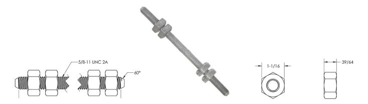
Double Arming Bolt 5/8" x 24" with 4 Nuts Hot dip Galvanized OFT-BDA5824, with 24 in Overall Length, 5/8 in Dia Rod, 24 in Thread Length, Steel, Hot-Dipped Galvanized and 47.25KN Tensile, are fully threaded and used in double crossarm construction to secure and lock in spacing between crossarms.
