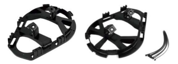
The fiber storage snowshoe clamp racket is an element for storing the cable reserve in the connections when aerial fiber optic installations are made. It can be placed directly on the ADSS cable without damaging it thanks to the included accessories.
