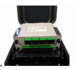
OTBL-0616L16AOHD2K is a plastic fiber optic terminal box that suitable for optical fiber splicing, distribution, and protection. Can load 1pc plastic splitter cassette 1x16. It supports 16 drop cable output and cable entry without cutting. SC/APC compatible, with reasonable bending radius for fiber protection. Allows outdoor cable splitting fusion.
