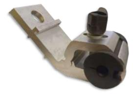
The mini-brackets are used for short and medium spans of ADSS fiber optic cables as well as Aerial Drop cables. Mini brackets are sized to fit specific ADSS diameters. Standard mini brackets are employed with fitted bushings to provide a good support/groove fit and to prevent the support from damaging the cable. The bolted supports are supplied with galvanized steel bolts to simplify installation with no loose parts.
