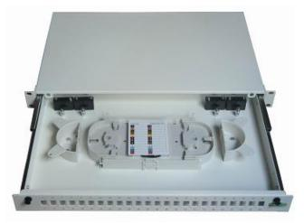
The Optical Patch Panel is made of cold-rolled steel inside, with plastic tray for pigtail cable distribution. Sliding drawer has aluminum sliding fittings with self-locking functions to prevent the drawer from falling during moving.
