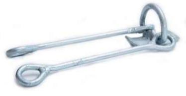
OFT-DCA 2A is made from hot-dip galvanized steel ASTM A-36 in accordance with ISO R 1460 and ISO R 1461 standards. Its minimum lengthening in 50mm is 21%. Its base is 50mm\*106mm with a tolerance of 10%. Hardware is designed to hold ADSS 120m span.
