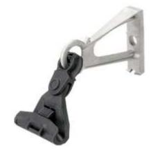
Suitable for insulated neutral 35, 50, 54 and 70mm2. Consist of glass fiber reinforced them -plastic UV resistant suspension clamp and a CS-14 aluminum alloy bracket which can be bolted with M12 or M16 bolts or strapped to the pole with 2 stainless steel straps 20mm\*0.7mm. It is delivered without bolt and straps.
