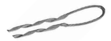
The OFT-PGG XXX preforms are made up of 5 powerful helical ASTM A36 steel wires to evenly distribute the gripping force and tension, their anti-corrosion process is based on the ASTM 123 hot-dip galvanized standard. The OFT-PGGXX is designed for the perfect anchoring of ADSS cables in the deployment of FTTX networks.
