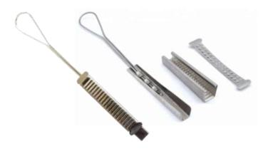
The OFT-CLSS DPC fitting is made of AISI 304 stainless steel to Warrant a long and useful life. The drop cable tension clamp is equipped with a perforated AISI 304 stainless Stel wedge, which increases the tension load preventing the cable from slipping without causing damage to the drop cable.
