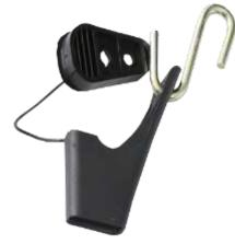
These anchoring clamps are made of one opened conical fiber glass reinforced body, a pair of plastic wedges and a flexible bail. Different sizes offer a wide range of gripping capacities and mechanical resistances to fit the various ADSS cable designs. The ADSS series of anchoring clamps allow an easy and quick securing of  $\emptyset$  6 to 20 mm aerial circular fiber optic cables (ADSS) on short spans (up to 150 meters).
