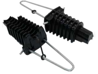
These anchoring clamps are made of one opened conical fiber glass reinforced body, a plastic wedges and a SS201 bail. The anchoring clamps allow an easy and quick securing of  $\Phi 8$  to 22 mm conductors.
