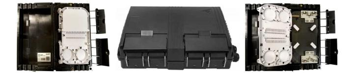
OSCH-24AH Fiber optic splice closure is made of high-quality ABS material. It is widely applied to the splicing and distributing variable optical cables. Features a compact structure, with rotary internal structure, super stratum for splicing and distributing, and substratum for cable arrangement. It also supports cable entry without cutting.
