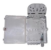
OTB 0608AOW Fiber optic terminal box is available for the distribution and terminal connection of various kinds of optical fiber system, especially suitable for mini-network terminal distribution, in which the optical cables, patch cords or pigtails are connected.
