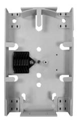
Fiber Optic Surface Box (Faceplate) supports up to Two SC adapters, for indoor domestic installations, easy-open box, which allows access to the cable entry and maintains a minimum radius of curvature appropriate for the installation of splitter, pigtail and Drop fiber.
