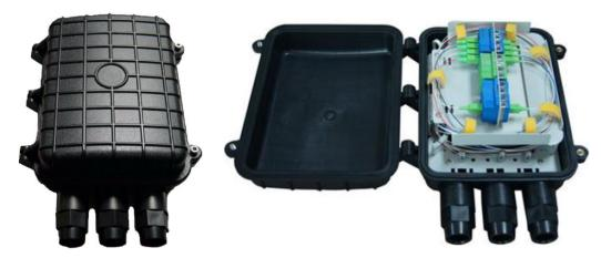
OSCH-24A is a small size fiber optic splice closure that is made of high-quality ABS material. It is used for fiber optic cable splicing and protection. The external component and fastening piece are all made of the high-quality steel. It can be opened after sealing.
