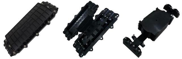
OSCH-120 has 4 fiber cable in-out round ports for diameter  $\Phi$ 7- $\Phi$ 18mm cable entry. It is widely applied to the splicing and distributing variable optical cables. It is made of ABS plastic and with the mechanical sealing structure filled with the sealing material. It can be opened after sealing.
