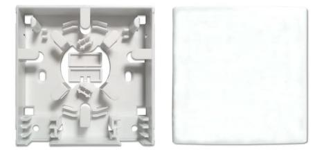
Fiber optic faceplate (Fiber optic wall socket) is used for end user indoor application. It's made of High-quality ABS plastic. Allows maximum 2pcs SC Simplex adapters. 2 fibers splice.
